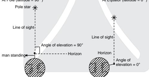
with the two pictures it is clear that latitude angle is equivalent to angle of elevation.
